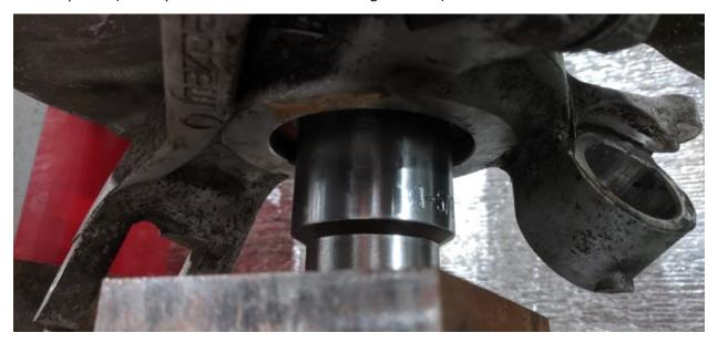
Reinstallation on the car is the reverse of removal. The spacer--the large machined washer--should install with the ID chamfer (angle cut surface) facing toward the CV. This angle provides clearance for the radius where the CV splines meet the body of the CV. The spacer should allow use of the Ford CV dust shield. This will run close to the Mazda knuckle but is not intended to touch when the CV is fully seated. Bearings are sealed so this a convenience rather than a requirement.
