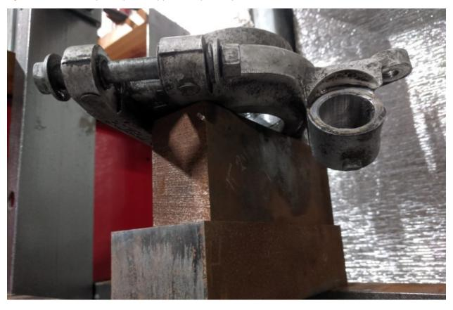
The old wheel bearing makes an idea driver to push in the new bearing. This ensures the press action occurs on the outer race of the bearing only.
