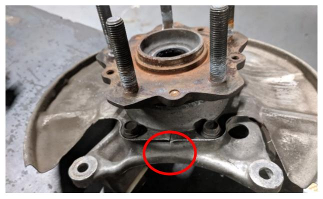
Press out the old hub using appropriately sized sockets or scrap to push on the hub only. Two sets of blocks in a crossing pattern may be useful to support the assembly. All thread not required but keeping things stable. A large bearing splitter could be useful here as well.
