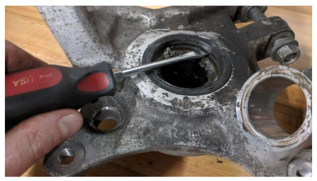
There is a large snap ring that retains the wheel bearing. Can someone grab a pic for us? It's shown here in the reinstalled configuration.
