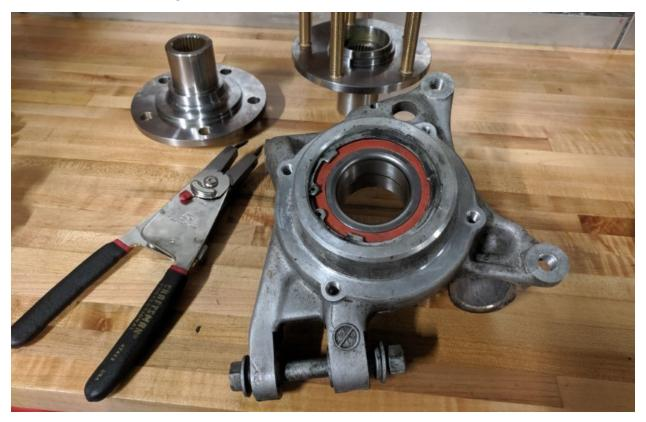
With the snap ring removed the wheel bearing can be pressed out. Ideally you'd like a very large socket such that you're pushing on the outside race of the bearing.
