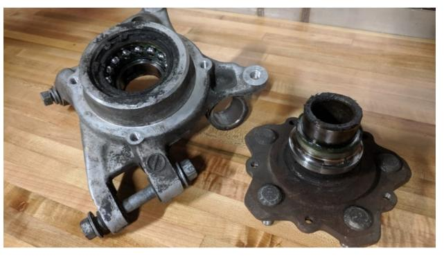
FCs used an inner CV seal not found on FDs. This seal will be removed and discarded using a flat screwdriver or pick. It will not be replaced on our final assembly.
