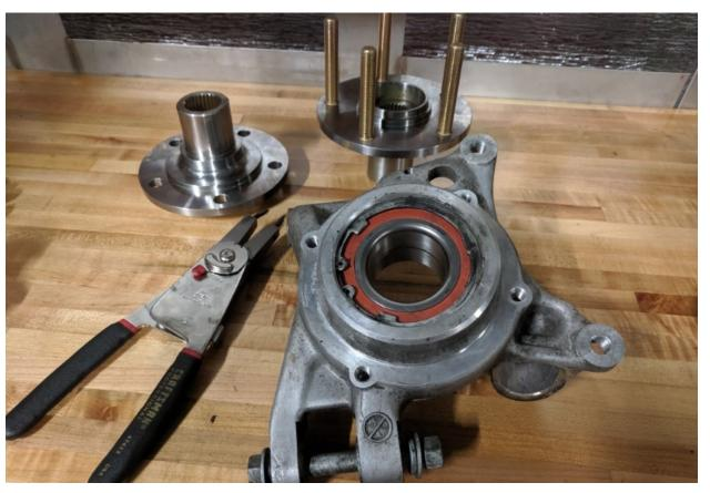
Dust shield is next and finally the hub w/ studs presses in place as an assembly. Lubing the bearing ID with a little grease is a good idea.
