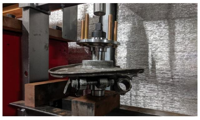
Note, you need to support the inner bearing race as the hub is driven through otherwise the bearing could separate (as likely occurred when the old bearing removed)
