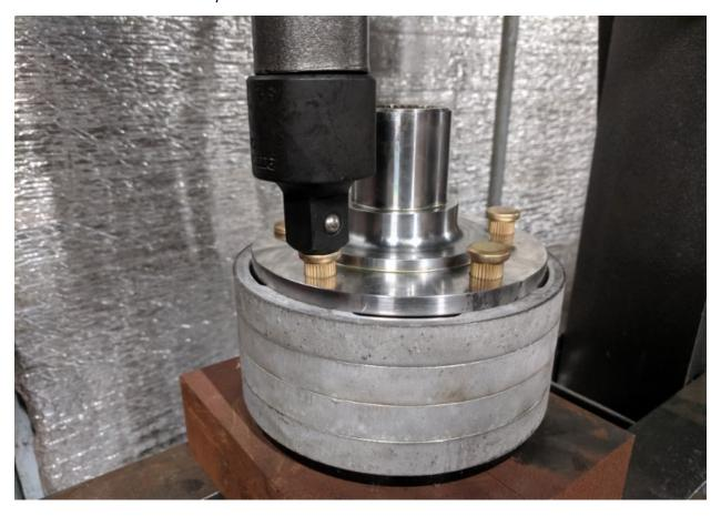
The wheel bearing is symmetric so either way is fine. A light coating of grease on the knuckle bore helps it run down smoothly.
