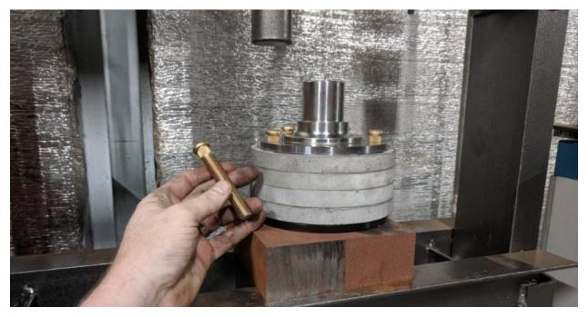
Drive the new studs all the way flush
