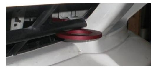
The front tow hook snakes through the bumper mouth so it can work on both s4 and s5 bumpers. Mounting uses flange bolts and ties to two factory threaded inserts on the bottom of the driver side frame rail. The spacer is included to drop the tow hook down slightly to clear the plastic cross bar on the s5 bumper.
