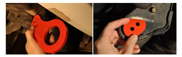
Rear tow hooks install with the "flats" opposite each other and bolts to the factory tow hook (works on either side). The flat at the back of the hook is vertical to clear a weld. The flat on the clamped part must be horizontal to clear a bend in the factory hook.
