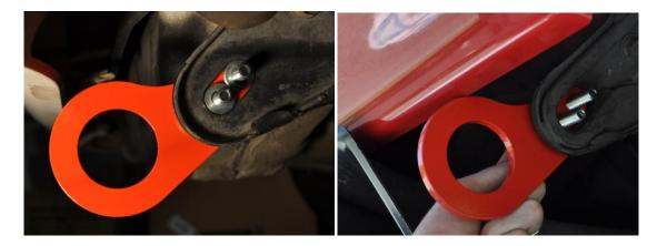
For s5 installations (shown above at left), 4 extra washers are provided to go inside the joint to help index the hook in the proper orientation. When used with an s4 (above right), longer hardware is provided and the internal washers need not be used.
